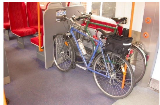
Cycle storage inside the doors of local trains: examples from Merseyrail and South Western Rail
