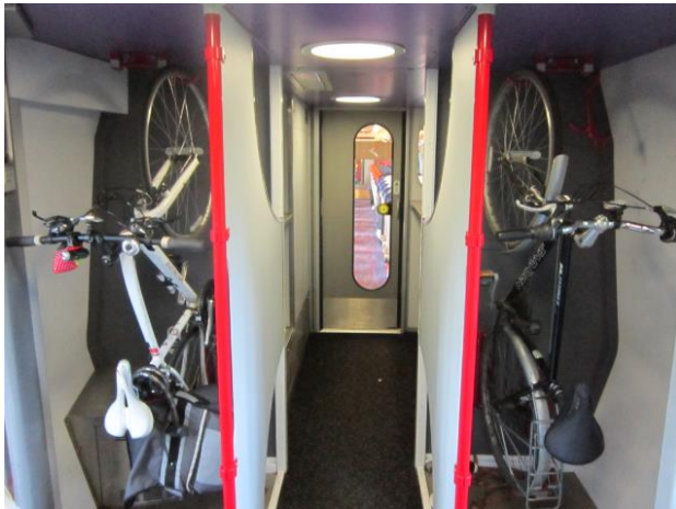
Bad practice from the UK: The Voyager and Intercity Express Programme (IEP) trains. Insufficient space, and very difficult to use – especially for shorter or disabled people – particularly when other passengers want to get past as the train leaves or arrives at a station.
