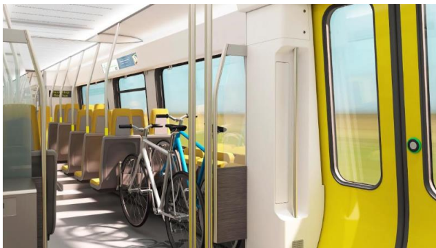
Cycle storage inside the doors of local trains: examples from Merseyrail and South Western Rail
