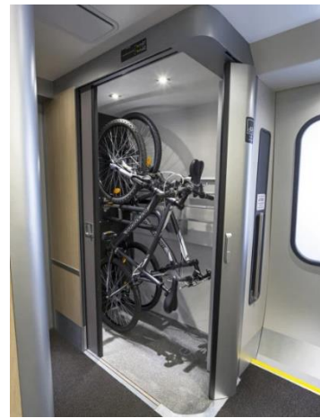
Bad practice from the UK: The Voyager and Intercity Express Programme (IEP) trains. Insufficient space, and very difficult to use – especially for shorter or disabled people – particularly when other passengers want to get past as the train leaves or arrives at a station.
