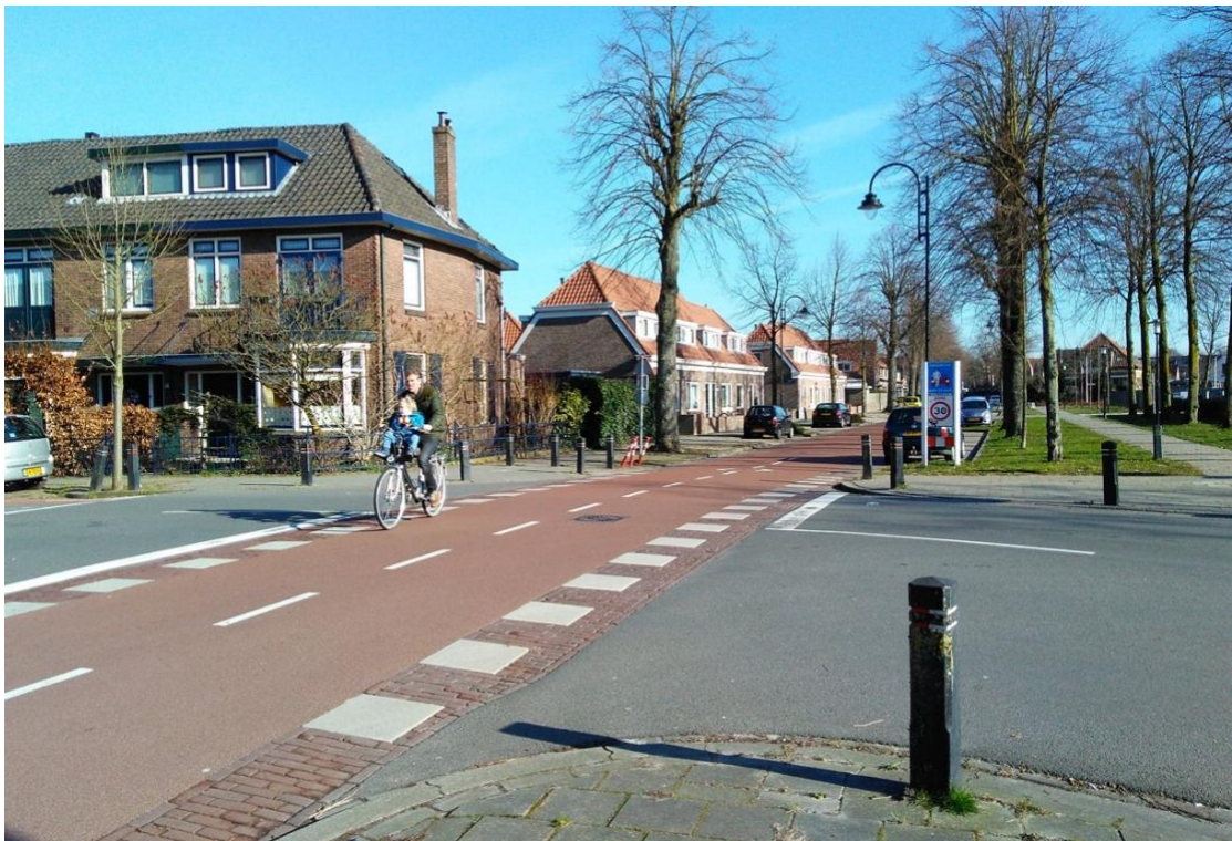
Figure 26 Cycle Priority Streets are widely used across the Netherlands and supported by a rule of no overtaking cyclists to support child road safety © J Read
