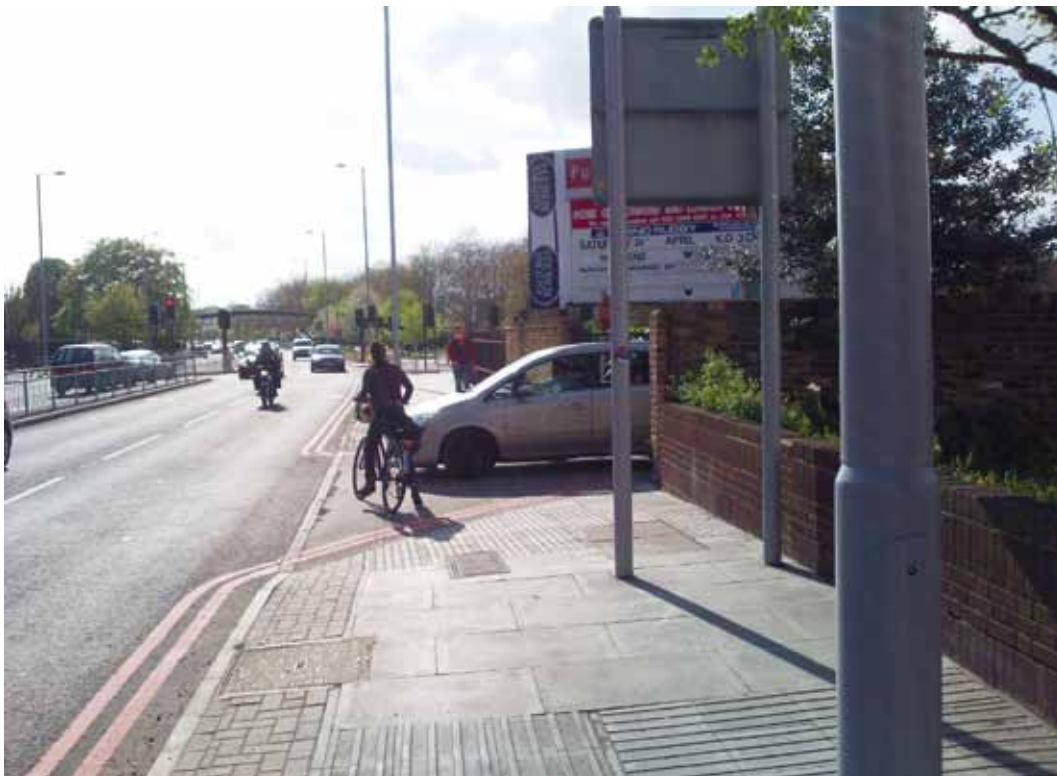
Figure 6.2 Potential for increased conflict where cycle track is two-way
