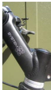
A threadless stem with a steep rise puts your handlebars higher
