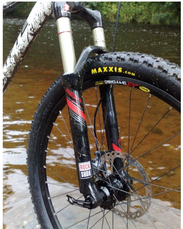
(Above and right) Fork and wheel will flex less in turns thanks to the oversize through-axle hub
