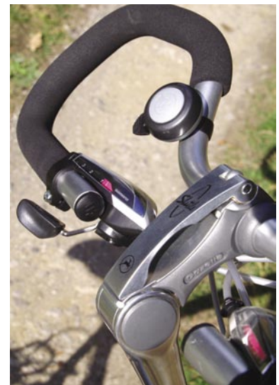
Gazelle's Shuttle QR stem makes it easy to adjust the angle and height of the Fuente's butterfly bar
