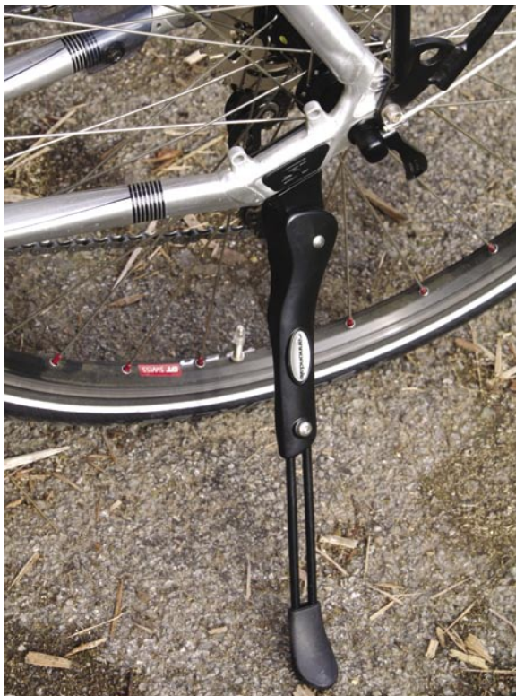
The Tesoro's extended rear dropout provides unobtrusive mountings for a stand and possible disc brake
