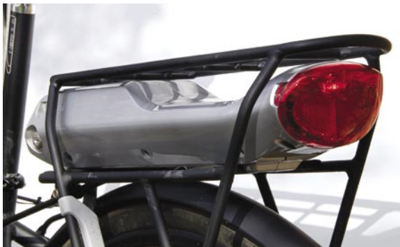
(Below) The Trek's battery incorporates a good rear lamp. (Bottom) The BionX control
