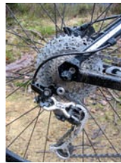
A cassette that goes to 36T compensates for the bigger wheels. The Fox fork (above right) has a reinforced steering response thanks to a tapered steerer and a 15mm axle. Its offset is 45mm
