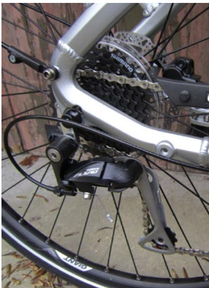
● (Above) The 9-speed 11-34 cassette on the Giant is as big as the Alivio derailleur is designed to cope with. For most users, that will be a sufficiently wide range, however, thanks to the extra motor power (up to 250W) available
