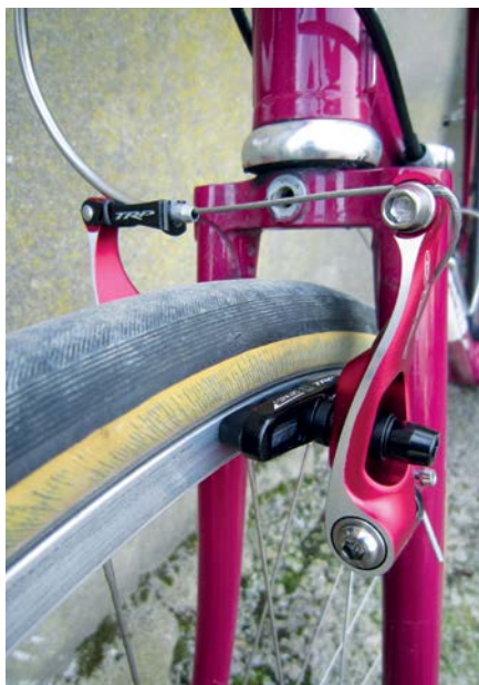
Above: Mini V-brakes are compatible with the shorter cable-pull of most drop bar levers
