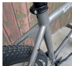
Above: The seatstays and chainstays are reinforced at the joints and equipped with mudguard and rack mounts
