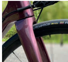
Top: An 11-32 cassette is fine, given the bike’s low weight Bottom: The full carbon fork underscores the Van Rysel’s sporty aspirations: it won’t take a conventional mudguard or a tyre bigger than 25mm
